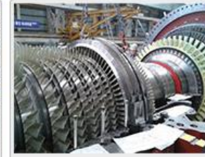
Blade Ring Assembly &amp; Clearance Check
