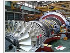
Blade Ring Assembly &amp; Bolt Tightening
